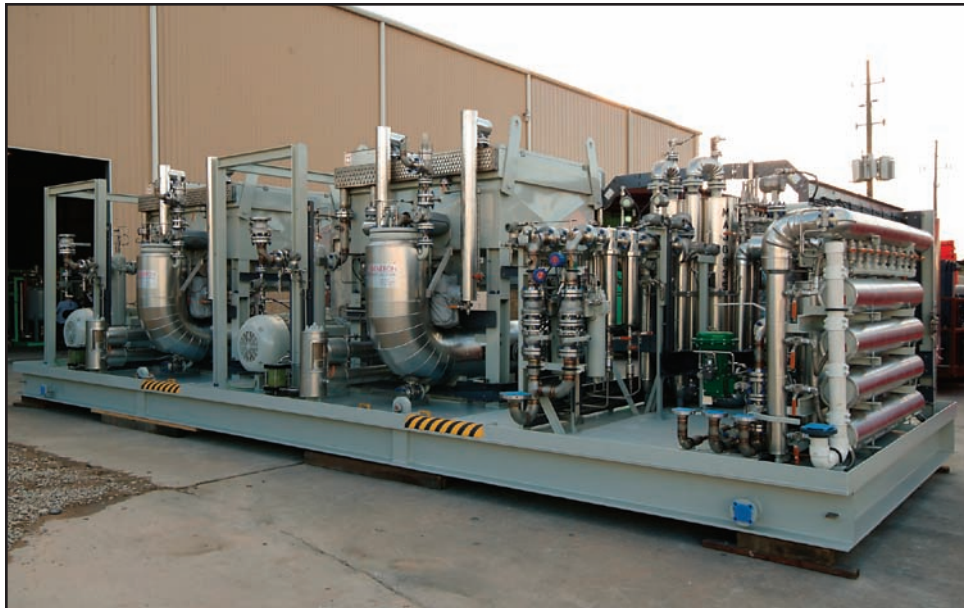
Hi-spec offshore instrument air and nitrogen plant with dual feed compressors.
